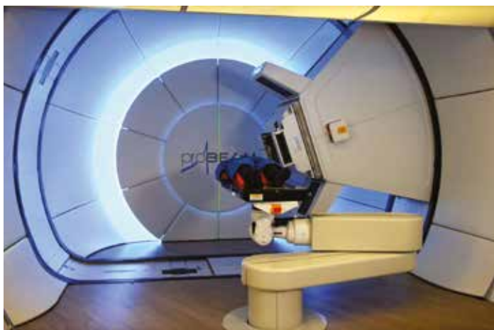
Proton beam equipment included three 360° treatment units and a 90 t super-conducting cyclotron shielded with 6 m thick walls
